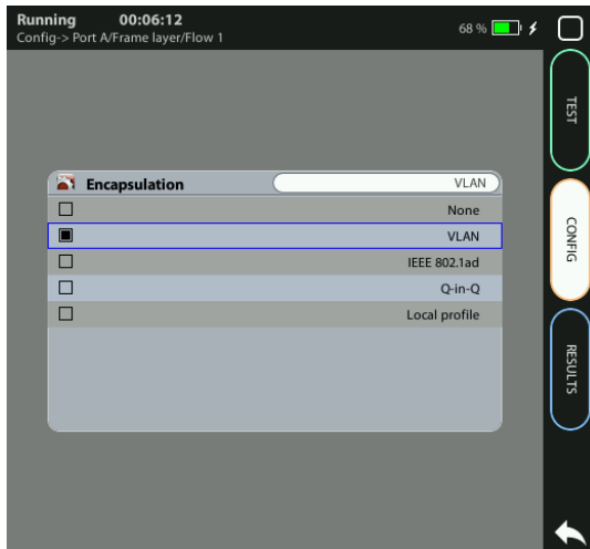
Figure 1.6: xGenius selection panel to enable users to choose between different Ethernet encapsulations
